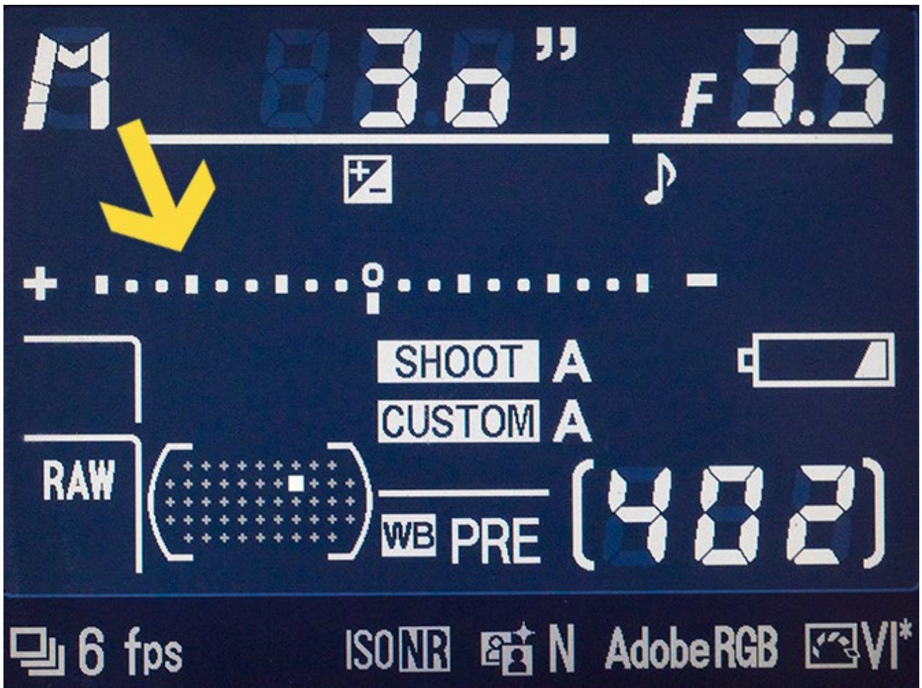
Screenshot of a camera LCD where you can see the light meter (+...0...-)
